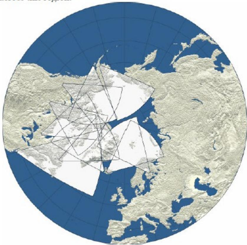
**Field-of-view of the SuperDARN network of coherent radars that exist in the northern hemisphere. A similar network exists in the southern hemisphere. This system monitors the electric fields.**
